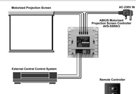
Works on momentary contract closure (dry contract, normally open, voltage free) only. Contact closure must set close for 1.5 seconds. (Warranty void if damaged is caused by inappropriate use.)
